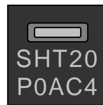
Figure 11 Laser marking on sensor. For details see text.
