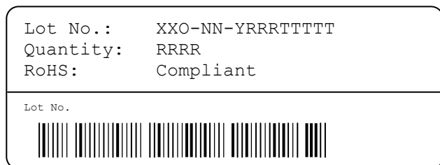
Figure 13: First label on reel: XX = Sensor Type (20 for SHT20), O = Output mode (D = Digital, P = PWM, S = SDM), NN = product revision no., Y = last digit of year, RRR = number of sensors on reel divided by 10 (200 for 2000 units), TTTTT = Traceability Code.
