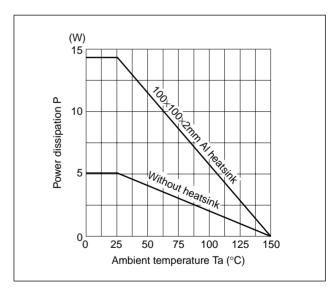
When selecting a heatsink for SLA5017, be sure to check the product temperature when in use in an actual applicaiton.
