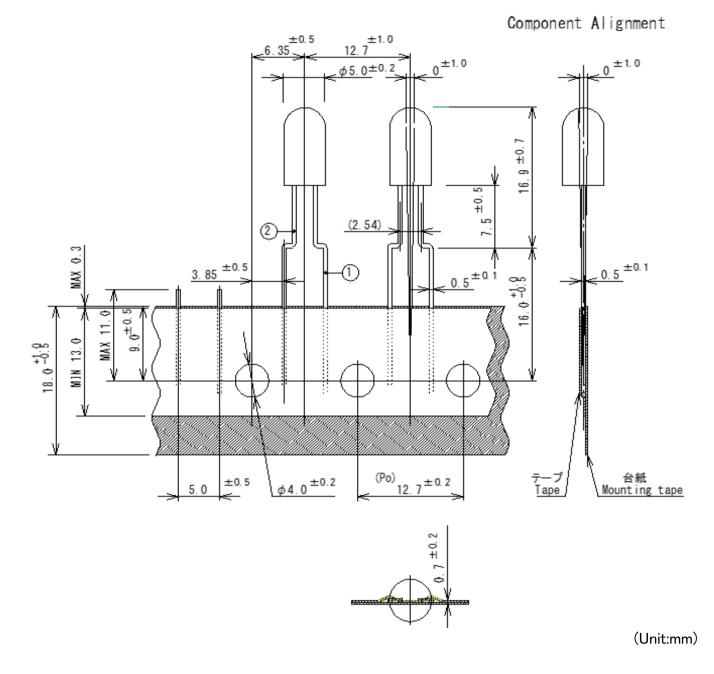
(Po):Accumulation pitch tolerance shall not exceed  $\pm 1.0$ mm over 20 consecutive pitches.
