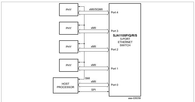
Figure 5. System diagram showing the SJA1105P/Q/R/S Ethernet switch connected to PHYs and a host processor. Port 4 is SGMII on SJA1105R/S
