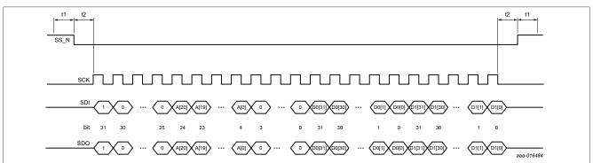
t1: The SPI slave select signal (SS\_N) must be stable for at least  $t_{d(W-R)}$  at the beginning or end of an SPI read or write operation before being asserted/de-asserted.
