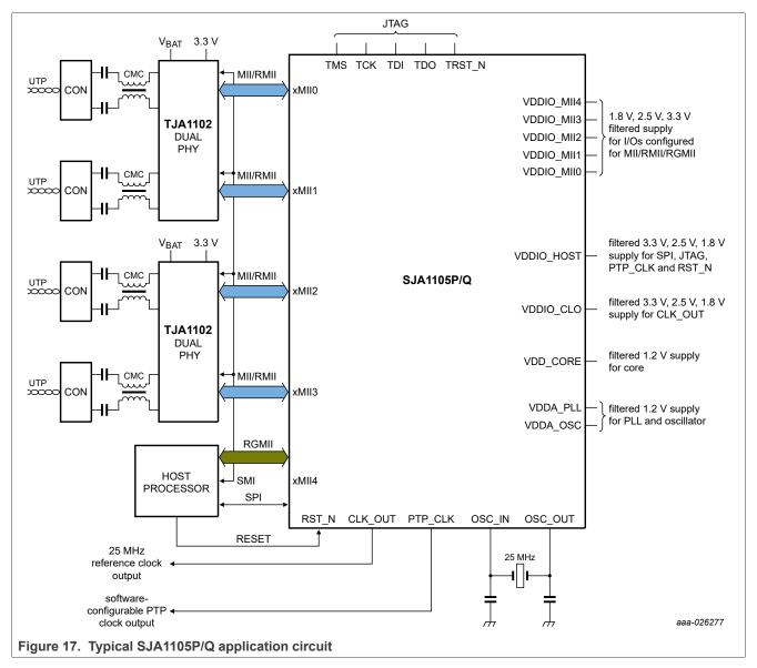
In this configuration, two TJA1102 100Base-T1 PHYs are connected to the SJA1105P/Q for MII/RMII operation while a host processor has RGMII connectivity with the SJA1105P/Q. For compatibility with the TJA1102, a VDDIO MIIx supply of 3.3 V must be selected.
