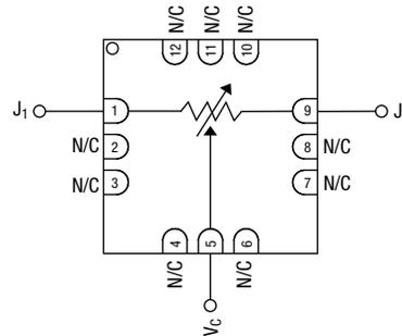
Ground is connected to paddle on bottom.
