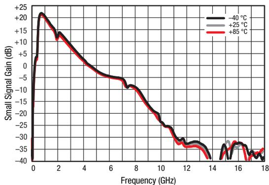
**Figure 3. Broadband Gain Response vs Frequency Over Temperature**
