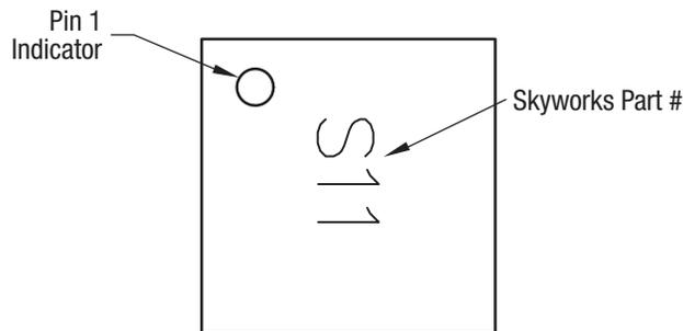
**Figure 27. Typical Case Markings (Top View)**
