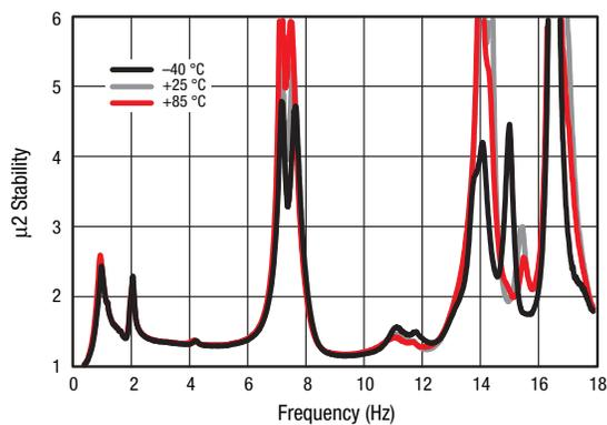
Figure 13. 2 Stability vs Frequency Over Temperature
