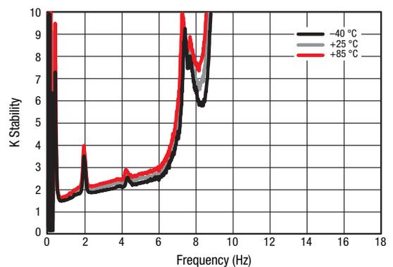
Figure 14. K Stability vs Frequency Over Temperature
