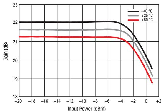
Figure 20. IP1dB vs Temperature (@ 700 MHz)
