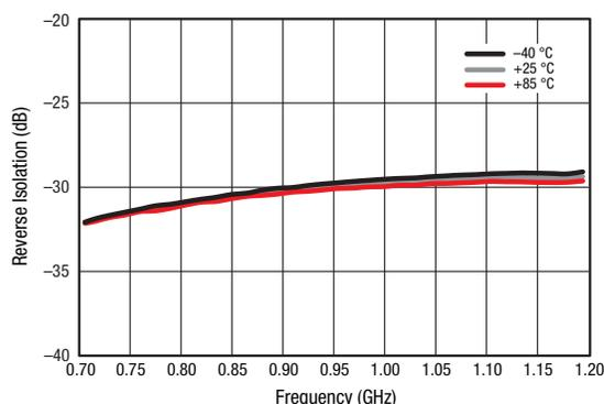
**Figure 8. Narrowband Reverse Isolation vs Frequency Over Temperature**
