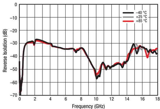
**Figure 7. Broadband Reverse Isolation vs Frequency Over Temperature**
