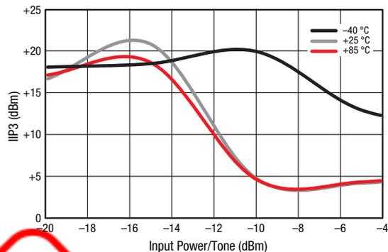
Figure 16. IIP3 vs Temperature (@ 700 MHz)
