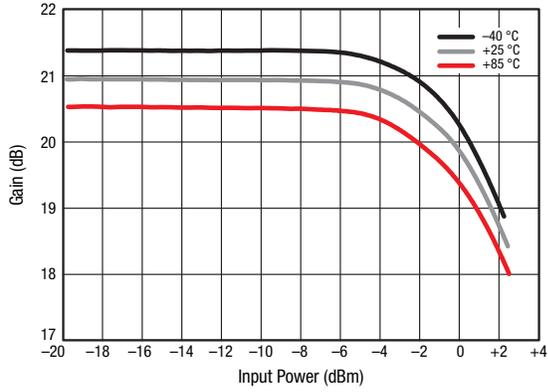
**Figure 21. IP1dB vs Temperature (@ 900 MHz)**
