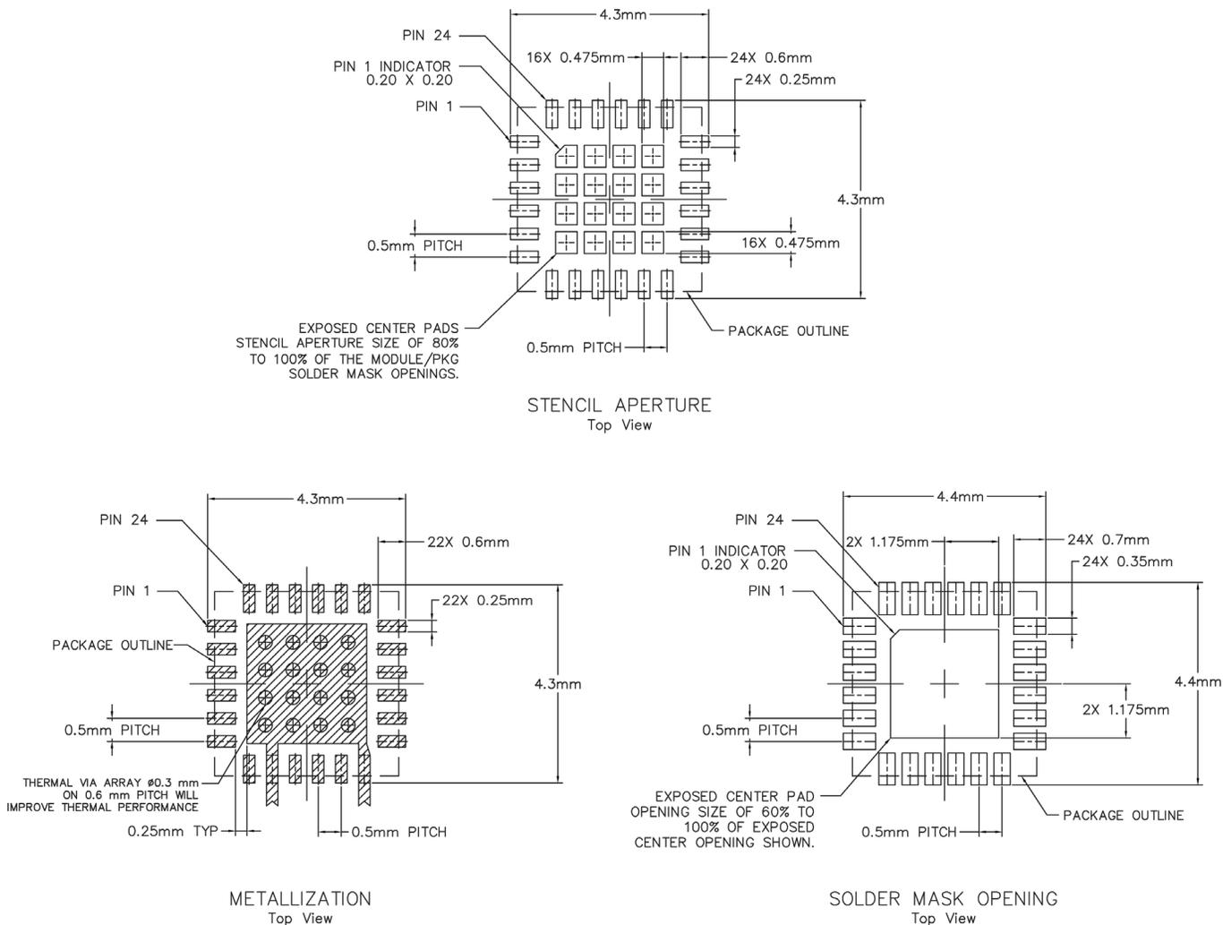
NOTE: THERMAL VIAS SHOULD BE RESIN FILLED AND CAPPED IN ACCORDANCE WITH IPC-4761 TYPE VII VIAS. 30-35UM Cu THICKNESS IS RECOMMENDED.
