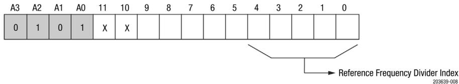
**Figure 8. Reference Frequency Dividers Register (Write Only)**
