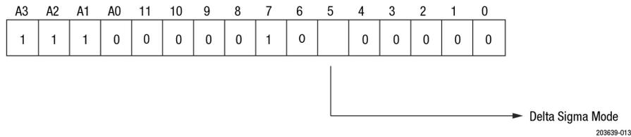
Figure 13. Delta Sigma Control Register (Write Only)
