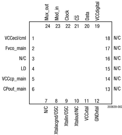
**Figure 2. SKY72310-11 Pinout (Top View)**
