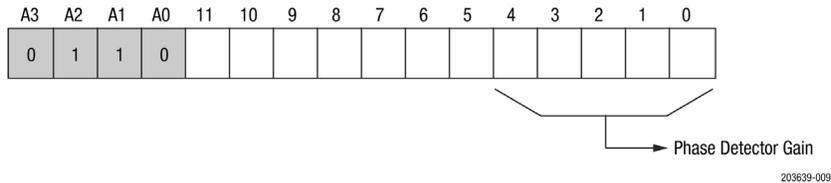
**Figure 9. Phase Detector/Charge Pump Control Register (Write Only)**
