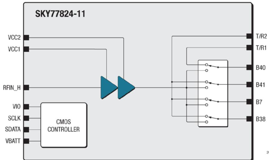
**FIGURE 1. SKY77824-11 FUNCTIONAL BLOCK DIAGRAM**
