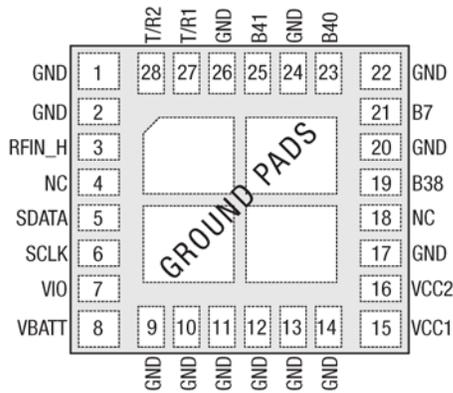
Pad layout as seen from Top View looking through package. GROUND PAD is package underside.
