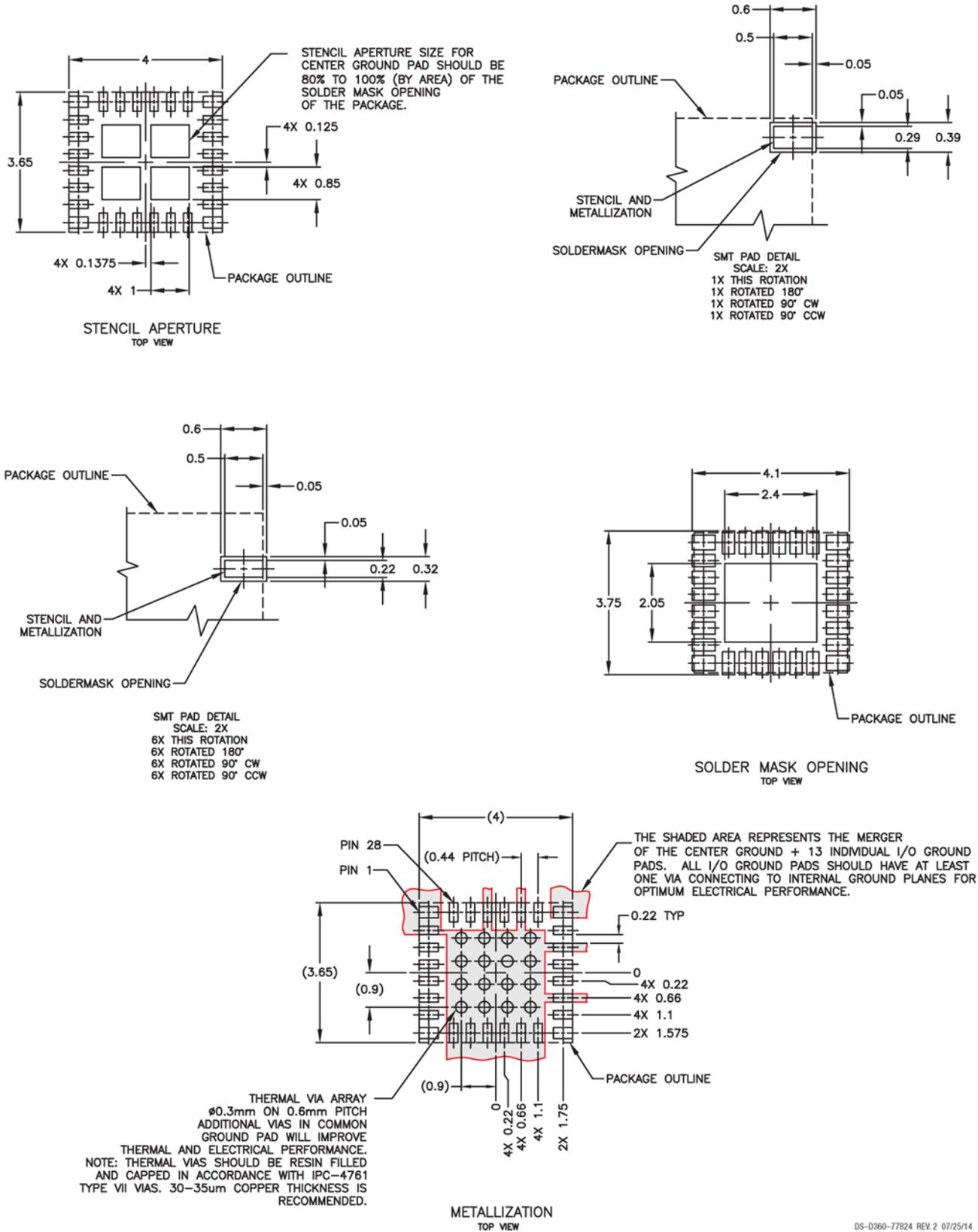
FIGURE 5. PCB LAYOUT DIAGRAM – 4.0 mm x 3.65 mm, 28-PAD PACKAGE – SKY77824-11
