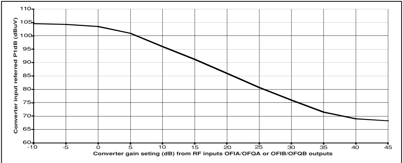
Figure 7. Variation in P1dB with converter gain (typical)
