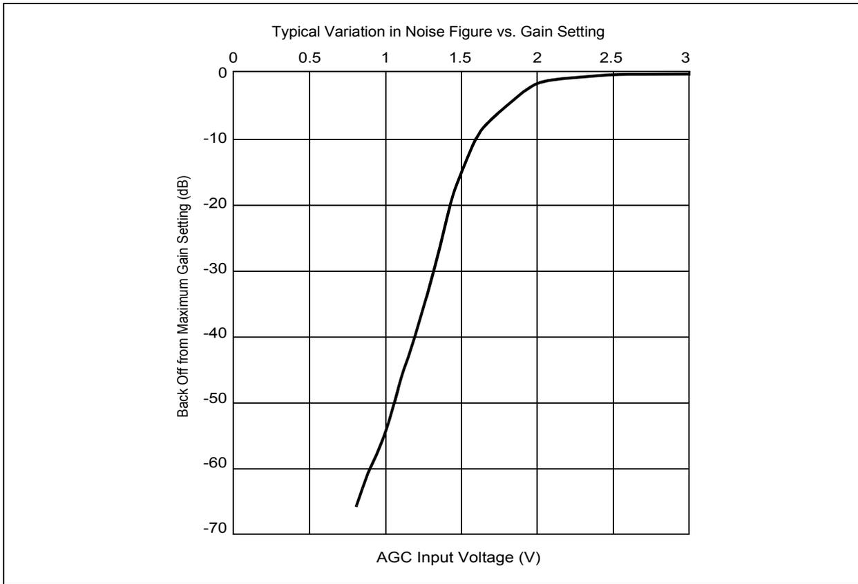
Figure 7 - Typical AGC versus Control Voltage Characteristic
