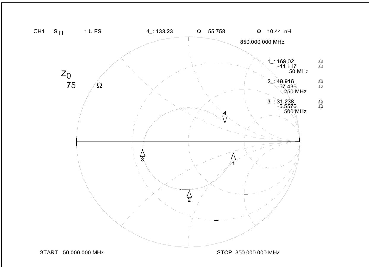
Figure 4 - Typical Single-Ended RF Input Impedance with Input Match
