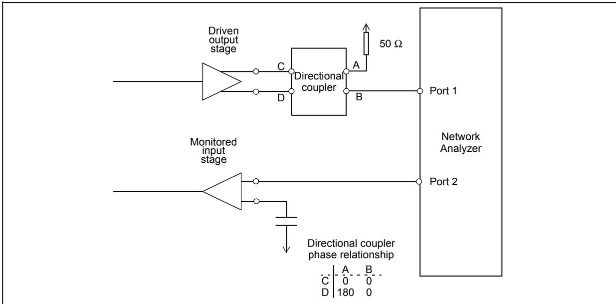
Figure 11 - Test Condition for Output to Input Crosstalk
