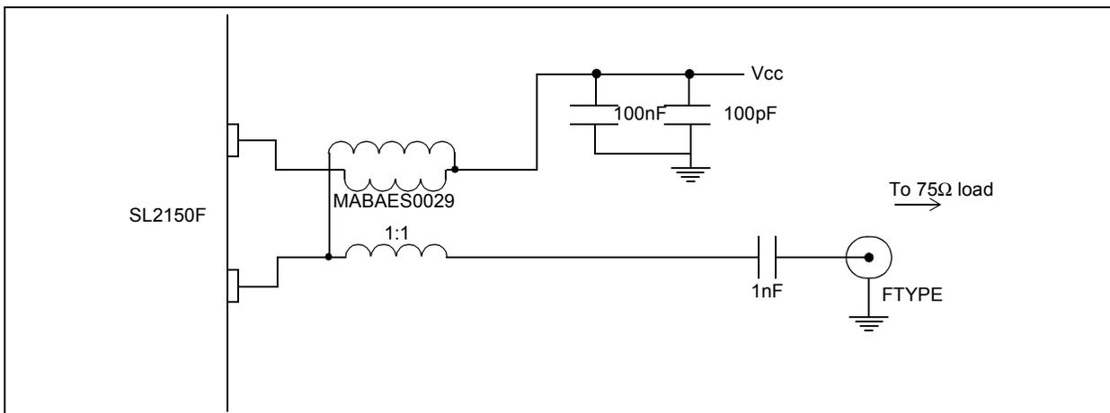
Figure 12 - Example Application Driving 75 Ohm Load
