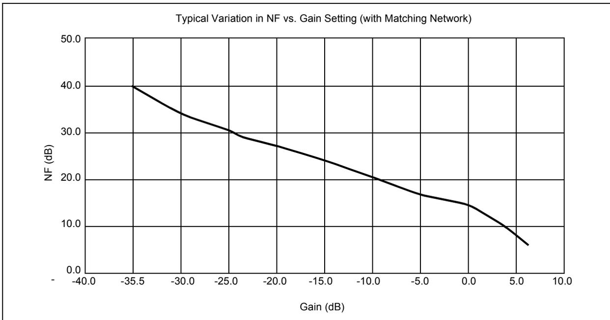
Figure 8 - Typical Variation in NF versus Gain Setting
