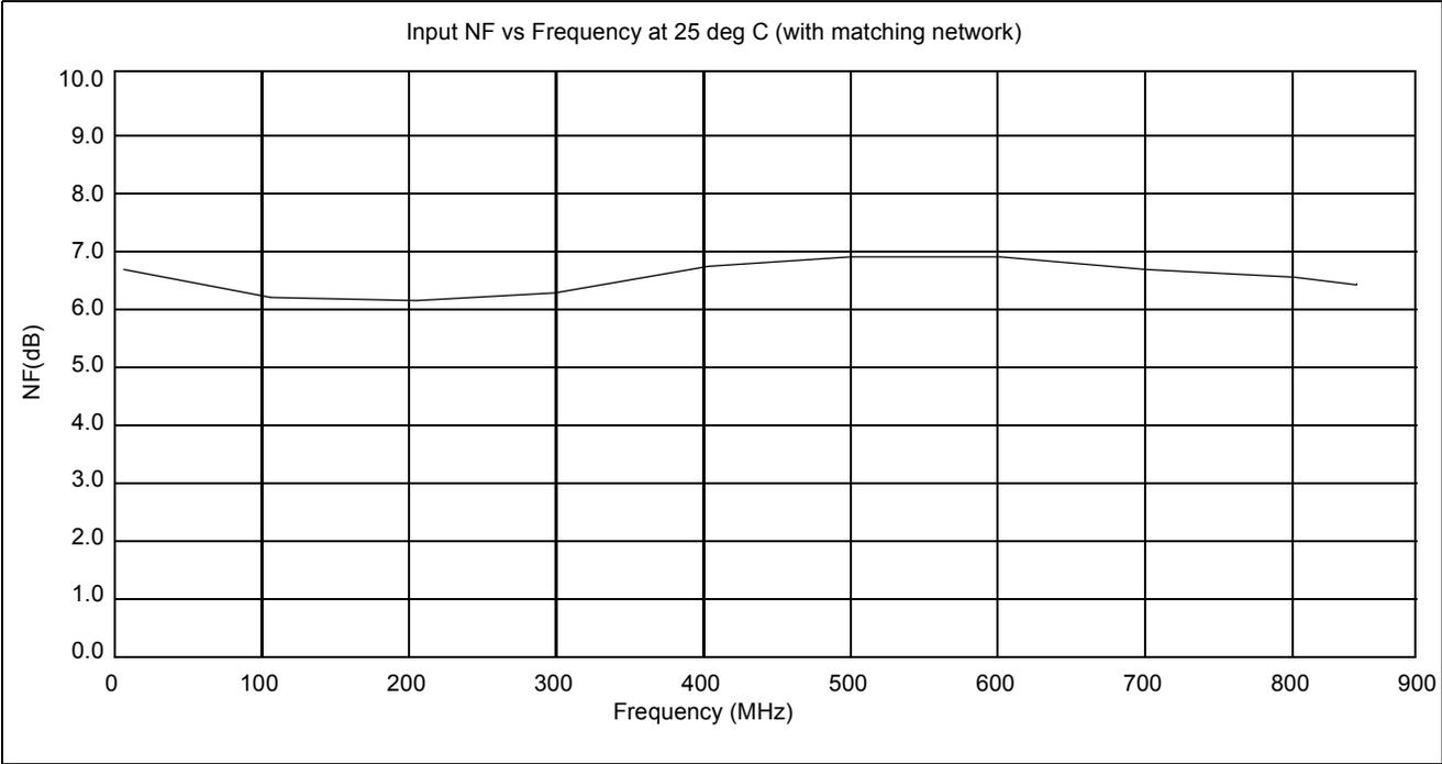
Figure 5 - Input NF at 25 deg C
