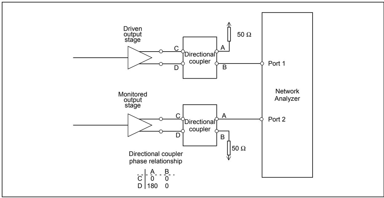
Figure 10 - Test Condition for Output Crosstalk
