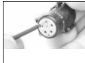
2. Insert a crimp terminated assembly into a selected cavity.
