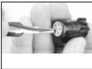
1. Open the CET - SLC Extraction tool and place it over the insulation of the wire.
