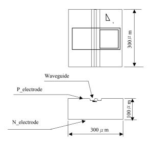
Bonding pad locate on the right side to the emitting direction.
