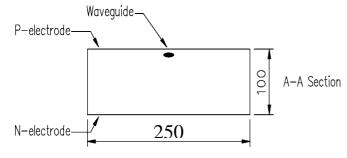
P-electrode and N-electrode are both gold pads.
