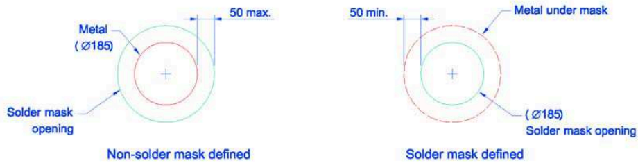
Solder mask detail (not to scale)
