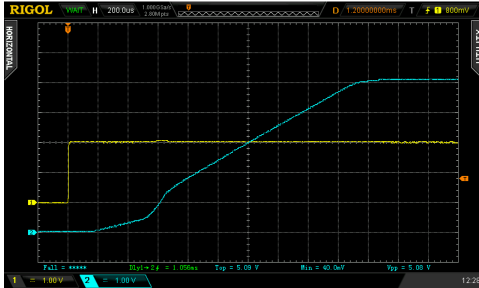
Figure 2. A SLG59M1717V with C_{SLEW} set to 4nF and 470 \mu F for C_{LOAD} . C_{LOAD} -to- C_{SLEW} ratio is greater than 33,600. Note that the internal SCL monitor's been triggered and V_{OUT(SR)} is reduced until V_{OUT} reaches \sim 0.25V.
