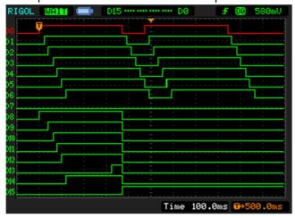
3. Sequencer after reset signal on PIN20 (FPGA\_PS\_RESET) operation
