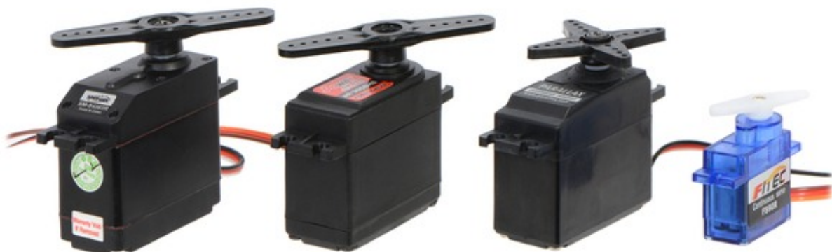
Continuous rotation servo size comparison. From left to right: SpringRC SM-S4303R, Power HD AR-3606HB, Parallax, and FEETECH FS90R.
