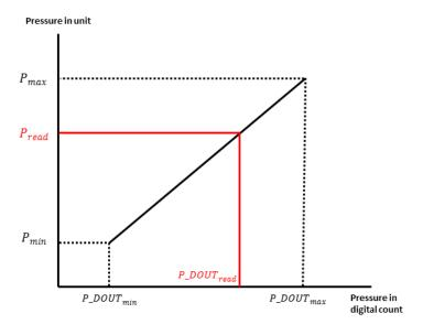
For example, the  $P_{min}$  and  $P_{max}$  for the sensor are specified as -15 psi and +15 psi. The  $DOUT_{min}$  and  $DOUT_{max}$  are -26214 and +26214. So,
