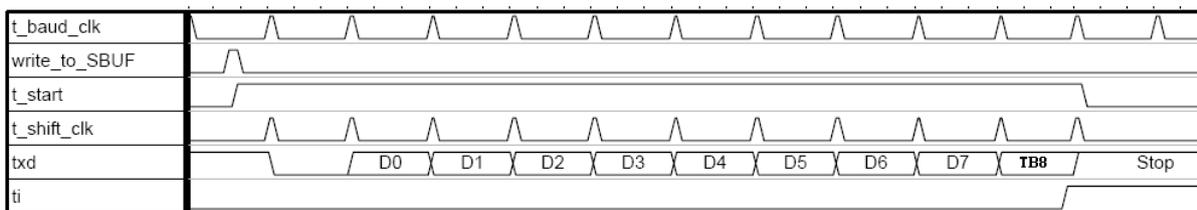
Fig. 7-5: Transmit modes 2 and 3 for Serial 0
