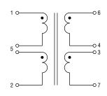
(Pin 1-2 & 6-7 / short 3-4) Turns Ratio (± 3 %) (Pin 1-2: 6-7 / short 3-4).....1:1 Insertion Loss (1-100 MHz) .....-1.5 dB max. Capacitance (Pin 5-3 / short 3-4) ......35 pF typ. Hi-Pot (Pin 1 to 6, short 3-4) Operating Temperature.....-40 to +85 °C Storage Temperature .....-40 to +85 °C Packaging ...... 2000 pcs. / reel
