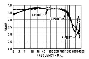
VSWR vs. Frequency: VSWR is the L-, l-, and R-ports in a 50 ohm system with  $f_L$  at +10 dBm. R- and l-port VSWR plotted with  $f_L$  at 1500 MHz.
