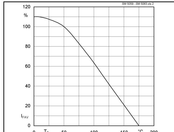
Fig. 2 Rated forward current vs. ambient temperature <sup>4)</sup>
