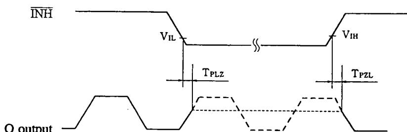
INH input waveform  $T_r = T_f = 10$  ns or less
