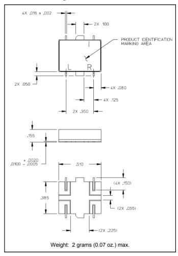
\* Dimensions are inches (millimeters) ±0.015 (0.38) unless otherwise specified.
