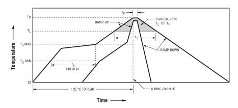
Ramp-up rate = 3 °C/sec. max. Ramp-down rate = 6 °C/sec. max.  $T_L$  = 217 °C  $t_L$  = 60-150 sec.  $T_p$  = 250 °C ±3 °C Time within 5 °C of actual Peak Temp ( $t_p$ ) = 20~40 sec.  $T_S$  min = 150 °C Ts max = 200 °C  $T_S$  min to  $T_S$  max = 60-180 sec. 25 °C to Peak Temperature = 8 min. max.
