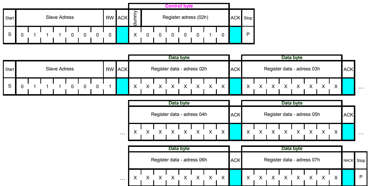
Figure 16: I 2 C multiple read protocol. Address register is first written to SMB380, the RW=0 (lowest acceleration data located at address 02h). I 2 C transfer is stopped and restarted with RW=1, address is automatically incremented and the 6 bytes can be sequentially read out.
