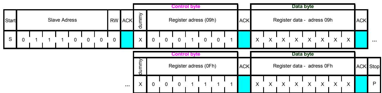
Figure 15: I 2 C multiple write protocol
