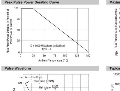
Peak Pulse Current (%) Pulse width (TP) is defined as that point where the peak current decays to 50 % of IPSM. 50 10 x 1000 waveform TA=25 °C as defined by R.E.A. ف TP 0-1.0 3.0 0 2.0 4.0 T, Time (ms)
