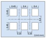
The recommended thickness of the screen mask for soldering is between 80 and 130 $\mu m$ . The hole size of the screen mask should be same as the recommended land pattern or smaller.
