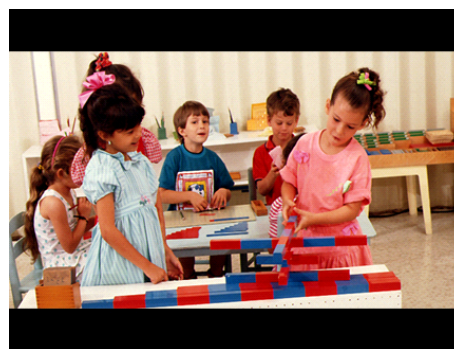
Figure 17-4 Scaling 16:9 content for a 4:3 display – “Letterbox” mode
