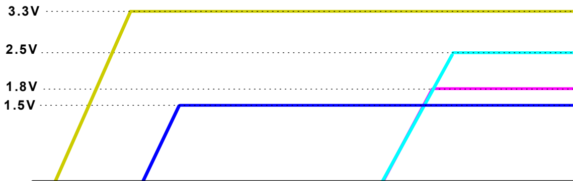
Figure 2A – Example Power Supply Sequencing and Tracking using the SMT4504. Any order of supply sequencing/tracking can be applied using the SMT4504.
