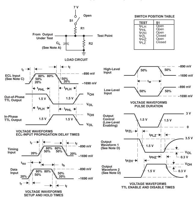
NOTES: A.C<sub>I</sub> includes probe and jig capacitance.
