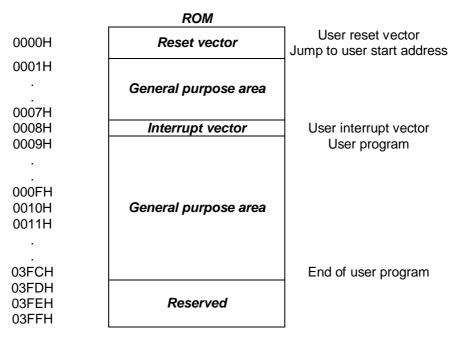
The ROM includes Reset vector, Interrupt vector, General purpose area and Reserved area. The Reset vector is program beginning address. The Interrupt vector is the head of interrupt service routine when any interrupt occurring. The General purpose area is main program area including main loop, sub-routines and data table.
