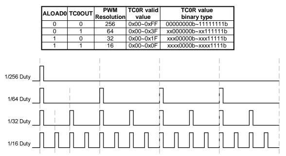
The PWM output pin is shared with GPIO and switch to output PWM signal as PWM0OUT=1 automatically. If PWM0OUT bit is cleared to disable PWM, the output pin exchanges to last GPIO mode automatically. It easily to implement carry signal on/off operation, not to control TC0ENB bit.
