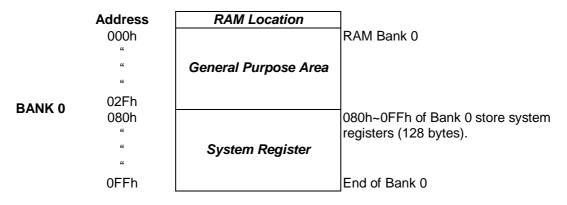
The 48-byte general purpose RAM is separated into Bank 0. Sonix provides "Bank 0" type instructions (e.g. b0mov, b0add, b0bts1, b0bset...) to control Bank 0 RAM directly.
