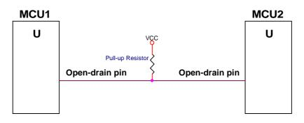
The pull-up resistor is necessary. Open-drain output high is driven by pull-up resistor. Output low is sunken by MCU's pin.
