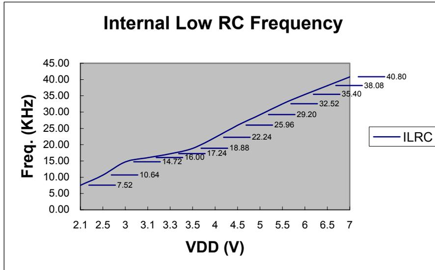
The internal low RC supports watchdog clock source and system slow mode controlled by CLKMD.
