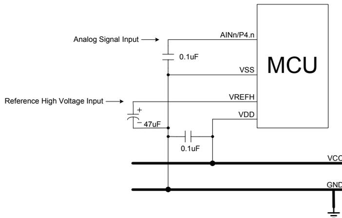
ADC reference high voltage is from external voltage and AIN0/P4.0 is VREFH input. The capacitor (47uF) between VREFH and VSS is necessary to stable VREFH voltage.
