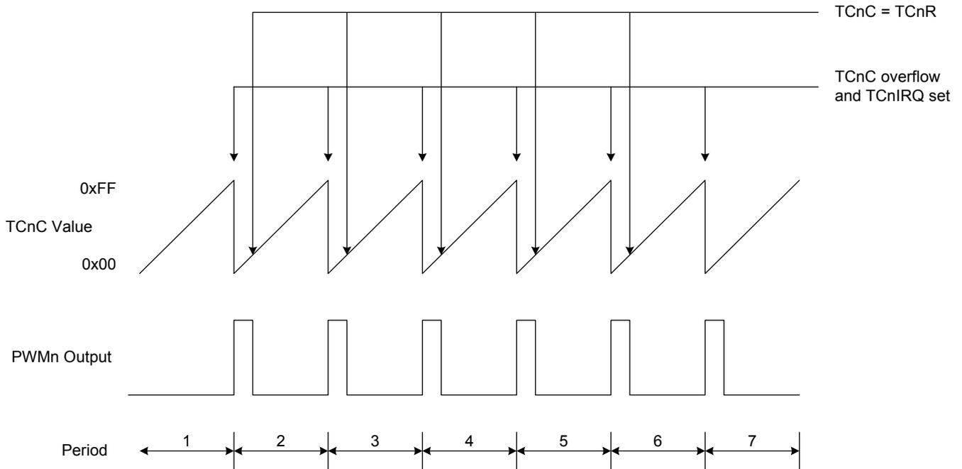
Above diagram is shown the waveform with fixed TCnR. In every TCnC overflow PWM output “High, when  $TCnC \geq TCnR$  PWM output “Low”. If TCnR is changing in the program processing, the PWM waveform will become as following diagram.
