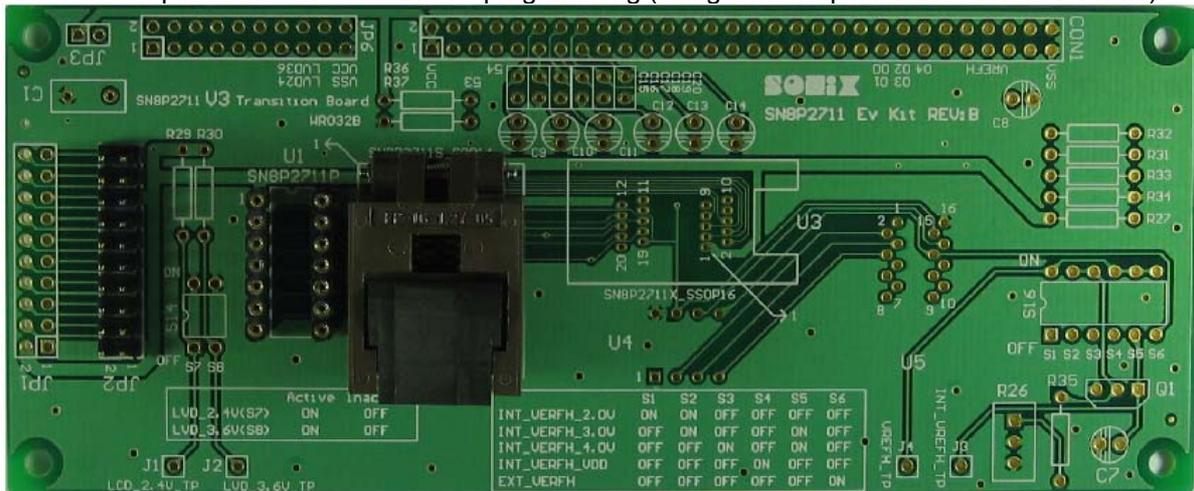
☞ **U3:** Set SSOP 16 pin socket for SN8P2711X programming (using SSOP 20 pin socket : **TX-SSOP20PIN**).
