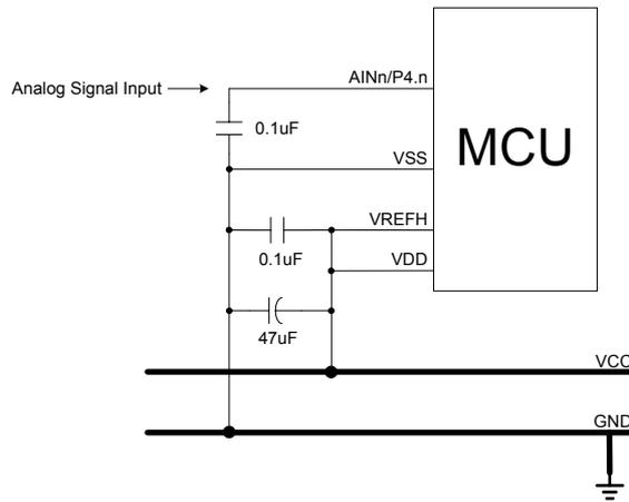
ADC reference high voltage is from VDD pin and AIN0/P4.0 is VREFH input. The VREFH should be from MCU's VDD pin. Don't connect from main power.
