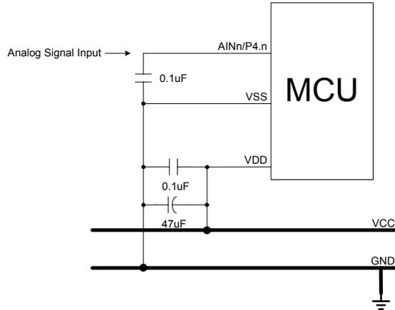
ADC reference high voltage is internal reference voltage and VREFH pin is AIN0/P4.0. The capacitor (0.1uF) between AINn/P4.n and VSS is necessary to stable analog signal.
