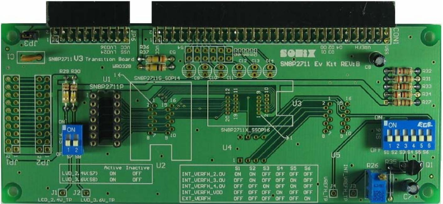
**CON1:** I/O port and ADC reference input. Connect to SN8ICE 2K CON1.
