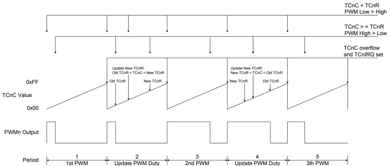
In period 2 and period 4, new Duty (TCnR) is set. TCn is double buffer design. The PWM still keeps the same duty in period 2 and period 4, and the new duty is changed in next period. By the way, system can avoid the PWM not changing or H/L changing twice in the same cycle and will prevent the unexpected or error operation.
