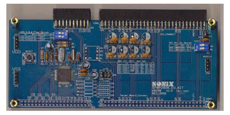
**CON1:** I/O port. Connect to SN8ICE 2K CON1.
