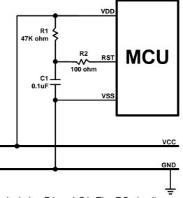
This is the basic reset circuit, and only includes R1 and C1. The RC circuit operation makes a slow rising signal into reset pin as power up. The reset signal is slower than VDD power up timing, and system occurs a power on signal from the timing difference.
