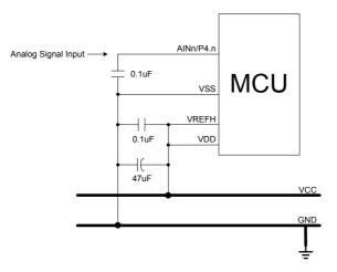
ADC reference high voltage is from VDD pin and AIN0/P4.0 is VERFH input. The VERFH should be from MCU's VDD pin. Don't connect from main power.
