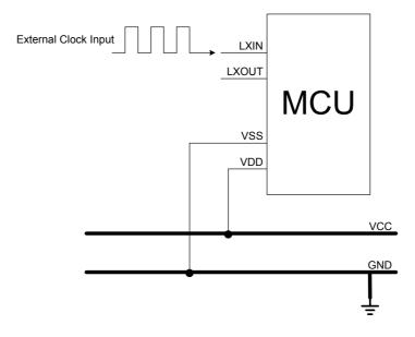
Note: The GND of external oscillator circuit must be as near as possible to VSS pin of micro-controller.
