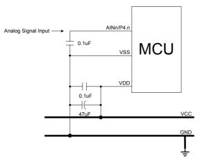
ADC reference high voltage is internal reference voltage and VREFH pin is AIN0/P4.0. The capacitor (0.1uF) between AINn/P4.n and VSS is necessary to stable analog signal.
