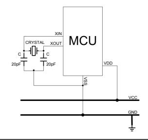
Note: Connect the Crystal/Ceramic and C as near as possible to the XIN/XOUT/VSS pins of micro-controller.
