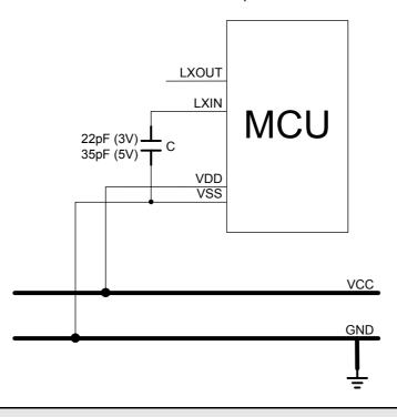
Note: Connect the C as near as possible to the VSS pin of micro-controller. The frequency of external low RC is decided by the capacitor value. Adjust capacitor value to about 32KHz frequency.
