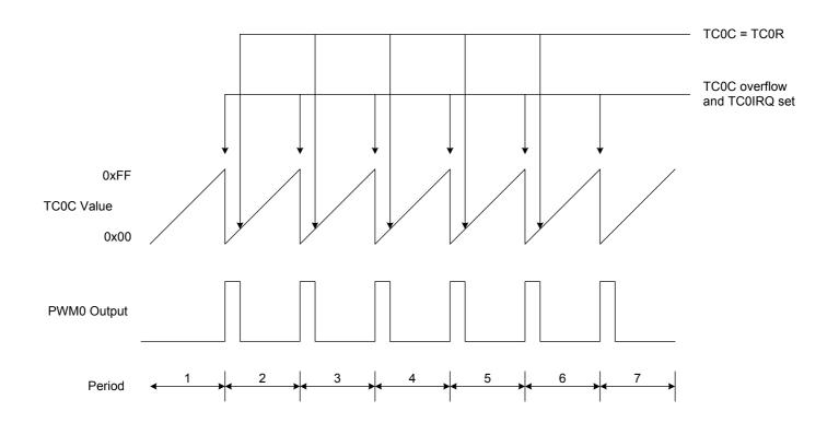
Above diagram is shown the waveform with fixed TC0R. In every TC0C overflow PWM output "High, when  $TC0C \ge TC0R$  PWM output "Low".
