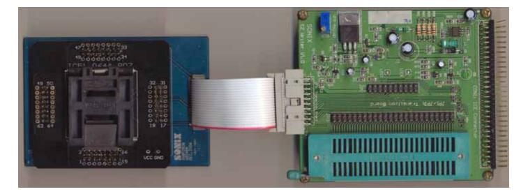
Note: Connect Easy Writer to ICE must be through an 60-pin cable
