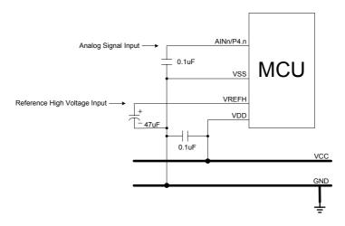
ADC reference high voltage is from external voltage and AIN0/P4.0 is VERFH input. The capacitor (47uF) between VREFH and VSS is necessary to stable VERFH voltage.
