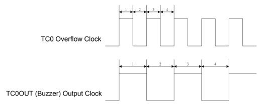
Example: Setup TC0OUT output from TC0 to TC0OUT (P5.4). The external high-speed clock is 4MHz. The TC0OUT frequency is 0.5KHz. Because the TC0OUT signal is divided by 2, set the TC0 clock to 1KHz. The TC0 clock source is from external oscillator clock. T0C rate is Fcpu/4. The TC0RATE2~TC0RATE1 = 110. TC0C = TC0R = 131.
