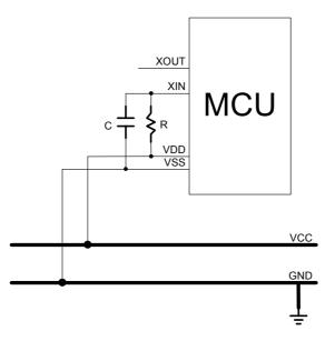
Note: Connect the R and C as near as possible to the VDD pin of micro-controller.
