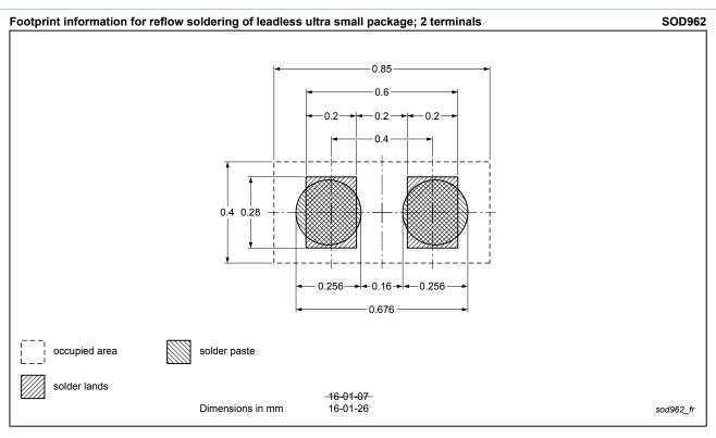
Fig. 2. Reflow soldering footprint for DSN0603-2 (SOD962)
