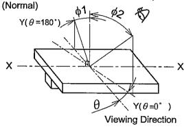
Note 2: Definition of viewing angle \$\phi 1\$ and \$\phi 2\$
