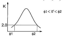
Contrast ratio K vs viewing angle  $\phi$
