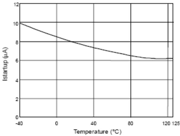
Fig. 9 Startup Current ( $I_{\text{startup}}$ ) vs. Temperature
