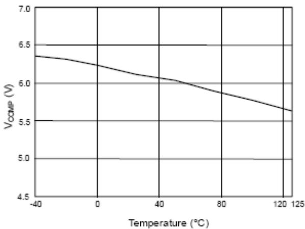
Fig. 11  $V_{\text{comp}}$  open loop voltage vs. Temperature
