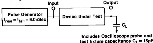
Includes Oscilloscope probe and test fixture capacitance C<sub>L</sub> = 15pF unless otherwise specified.
