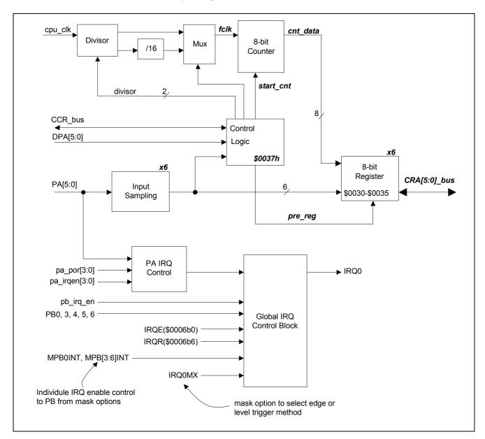
The start bit is designed to enable the operation. When the start bit is enabled and at least one of the DPA[5:0] is set to input mode, the counter starts counting up. When the counter reaches the value "FFh", it will keep the value until the start bit is cleared. Once the related PA port input is sampled from low to high, the count value will be stored into the related register. The data will be kept until the start bit is cleared.
