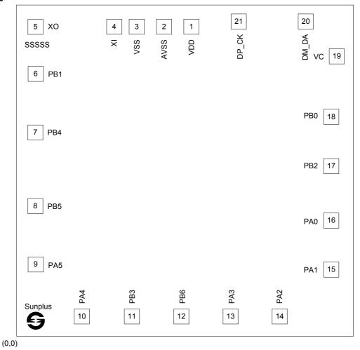
Chip Size:  $1740\mu m\ x\ 1770\mu m$  This IC substrate should be connected to VSS
