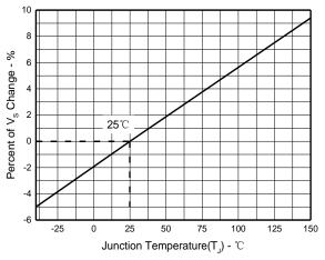
Normalized V<sub>S</sub> Change vs. Junction Temperature
