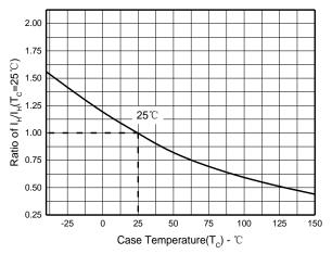
**Normalized Holding Current vs. Case Temperature**
