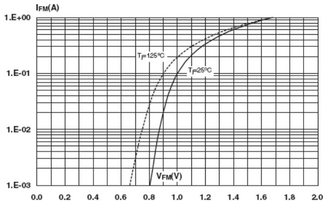
Fig 4 : Forward Voltage Drop V.S Peak Forward Current
