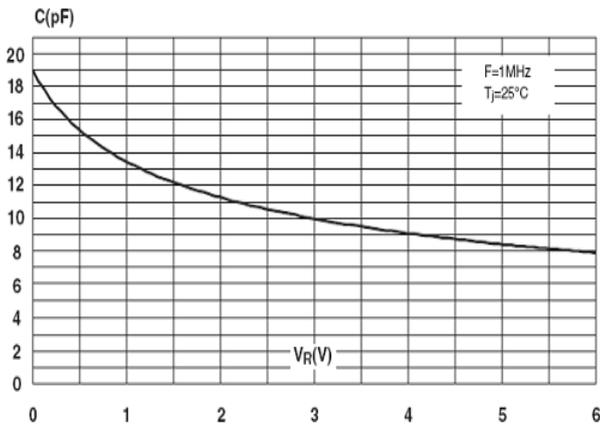
Fig 1 : Junction Capacitance V.S Reverse Voltage Applied
