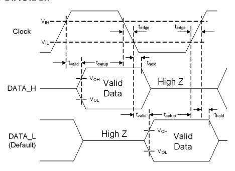
$$T_{clock}/2 = T_{edge} + T_{valid} + T_{setup}$$
