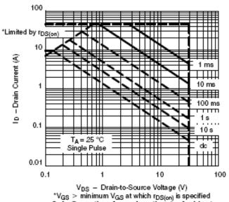
\*V<sub>GS</sub> > minimum V<sub>GS</sub> at which r<sub>DS(on)</sub> is specified Safe Operating Area, Junction-to-Ambient
