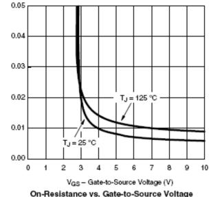
urce-Drain Diode Forward Voltage On-Resistance vs. Gate-to-Source Voltage
