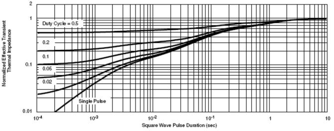
Normalized Thermal Transient Impedance, Junction-to-Foot
