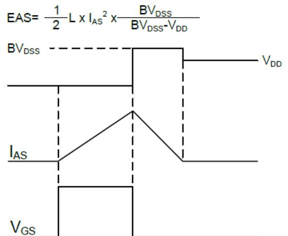
Fig.11 Unclamping Inductive Waveform
