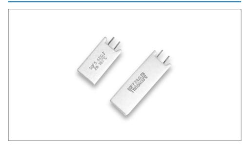
As the Thermal fuses are incorporated, these cement filled resistors respond quickly to overloading as well as to external overheating. The SQF series also provides outstanding features against surges, and are therefore suitable for the preventing of inrush current for switching regulators. Obvious economic advantages can be achieved by not having to specify a separate thermal fuse.
