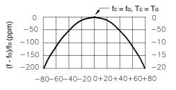
$\Delta T=T_{c}-T_{0} \ (^{\circ}C)$ The curve shown above accounts for resonator contribution only and does not include oscillator temperature characteristics.
