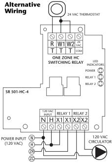
**NOTE:** When using Alternative Wiring diagram, the boiler operating control's ZC terminal will see the load of the circulator(s).
