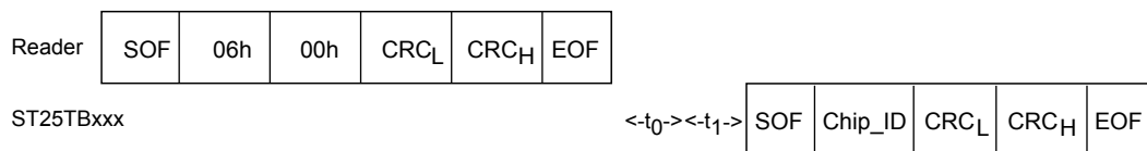
Figure 20. Initiate frame exchange between reader and ST25TB512-AC
