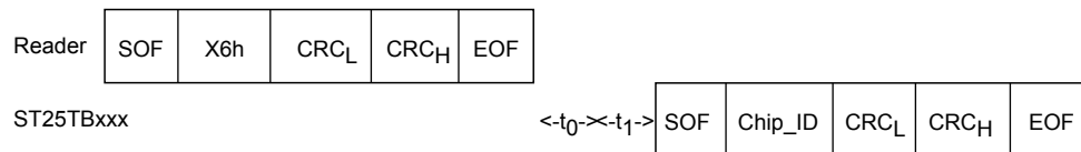
Figure 49. Slot_marker frame exchange between reader and ST25TB512-AC
