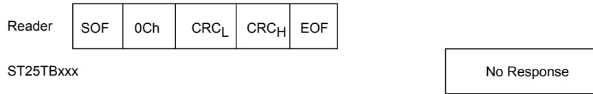
Figure 52. Reset_to_inventory frame exchange between reader and ST25TB512-AC
