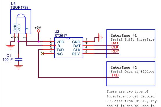
Interface #1 is Serial Shift Interface, which consist of three pins. In this interface you have to monitor RDY pin to go low which means new RC5 data has arrived. Then you shift output data using DAT and CLK pins. You can use any I/O of your application microcontroller.
