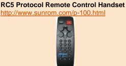
The 3rd bit is a toggle bit. This bit is inverted every time a key is released and pressed again. This way the receiver can distinguish between a key that remains down, or is pressed repeatedly.
