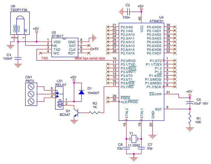
IMPORTANT: In serial data mode, the CLK pin#6 has to be connected to +5V to get data from TXD pin as shown above.
